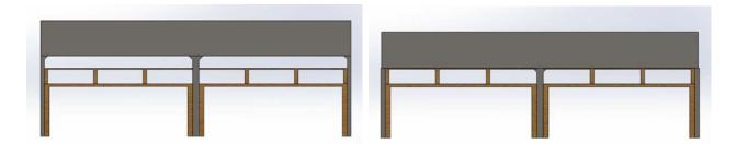
Figure 2. Conveyor height reduction from the original (left) to the final (right).
