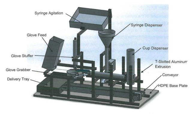
Figure 3: CAD Model of Full Packaging Assembly
