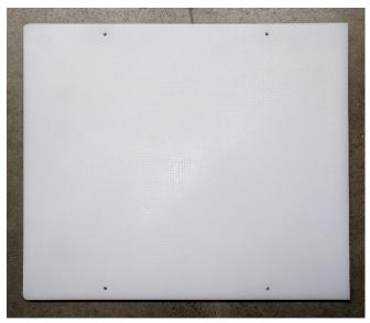
Figure 5. Cutting board cut to length with indexing holes.
