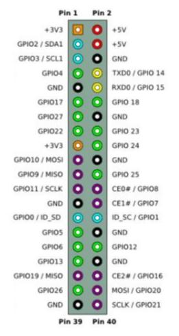
Figure 11: GPIO pinout diagram for Raspberry Pi
