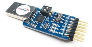
Figure 3: USB to Serial Converter
