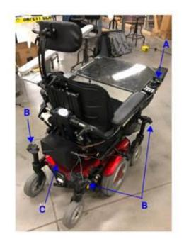
A: LED Indicator B: LiDAR Sensors C: Housing Box D: Battery E: Raspberry Pi F: Big7 G: USB to Serial Converter
